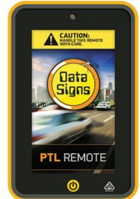
To enter a Demand for either Red or Green signal phase, press the **STOP** or **GO** buttons. On each Demand, the DEMAND LED's will flash to indicate a demand on the Master or the Slave. Refer to previous sections regarding comprehensive use of the Remote Control in various operational modes.
