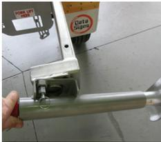
2. Always fully pull out the rear Jackstand Extenders. Wind down all four Jackstands to level the trailer. Raise to allow the wheels to spin freely, which stops the unit moving in windy conditions. A drill adaptor bit for the quick setup of Jackstands is also supplied.
