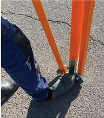
Push with your feet on the levers to allow the stabilizer feet to fall downwards.
