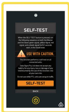
When the SELF TEST button is pressed, the following sequence is run on the PTL Compact to test the aspects, on any connected units:
