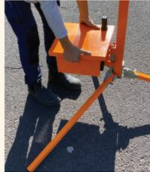
Align the notches in the control box over the metal bracket and lower onto it.
