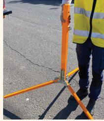
Once all feet are down, pull the center post upwards to lock each foot into place.
