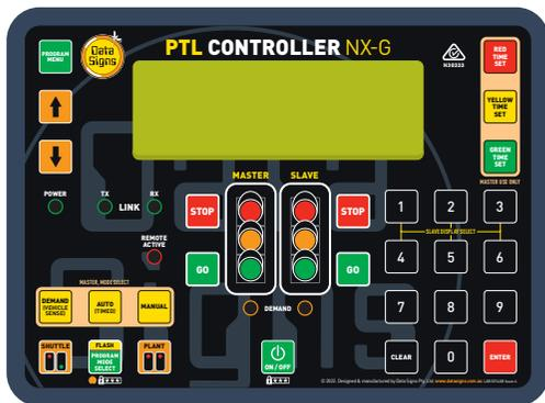
To switch the controller on, press the ON/OFF button
