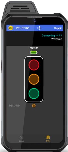
As the Bluetooth connection is established a progress sequence of 5-stars will appear, and the screen will redirect to the relevant remote screen.
