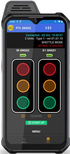
Your PTL Remote is normally set to pair to the Master PTL on startup, or see '*Switching ON and PAIRING the Remote*'.
