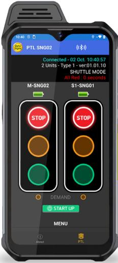
A demand for Green or Red signal on the Master or Slave is entered on the Remote Control unit. For Shuttle Control, on start-up, both the Master and Slave will rest on Red until a demand for Green is entered.
