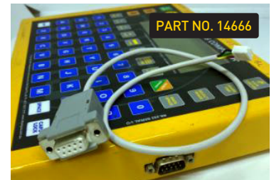
Adaptor for old style keyboard. Use VELCRO to hold keyboard on shelf. Plug adaptor in when needing to use the keyboard.
