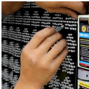
If maintenance on the LED boards is required, the T tool can be used as shown to unclip the board holder.
