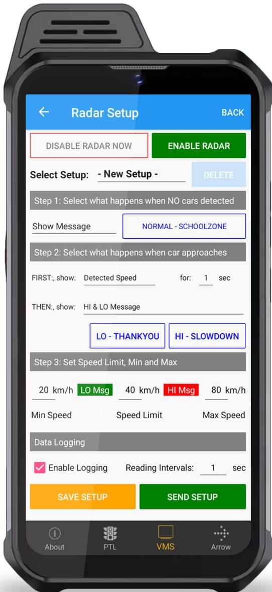
Start by tapping the **ENABLE RADAR** button.
