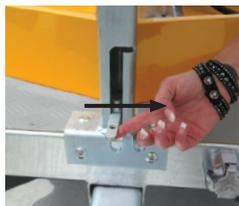
3. Lift the pin and move right to hold in up position, push the drawbar inwards until nearly all the way, then move pin handle back to the left and push the drawbar fully in, the pin will then drop into place again.
