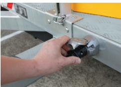
5. Undo the trailer cable and store this under the shelf in the VMS Control box.
