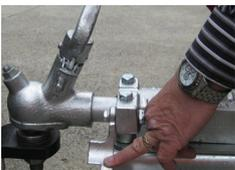
6. Note: when towing, ensure the reverse-lock is not engaged. Push out of the way, as shown.
