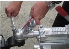
5. Tighten the locking nut firmly.
