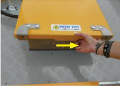
1. Raise the lid of the VMS Control Box by sliding the concealed latch underneath the lid to the right.
