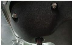
4. Insert the M6 TOOL BIT in **10mm past the cover screw thread section** and begin winding down the actuator **SLOWLY!** Otherwise there is a potential risk of electricity being generated as it winds and may damage the actuator.
