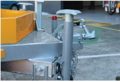
7. Pull the spring pin and rotate the wind-down legs upside down, ensuring the spring pin goes back in to lock.
