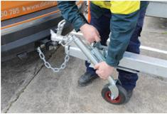
10. Wind up the jockey wheel and lift to slot into position. Make sure the jockey wheel does not move once in the towing position.
