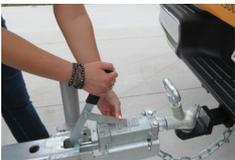
12. Release the hand brake if this is still engaged.
