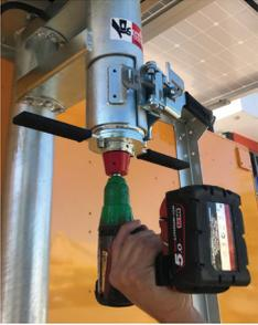
**CAUTION:** Failure to release the mast brake will cause damage to the mast brake or actuator.
