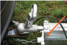
11. Ensure the Reversing lock on the tow coupling is released before travelling, as shown.
