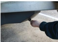
6. To drain the water, **first open the ballast tank caps.** Then use the plugs located at the bottom of each tank. There are two plugs on the front ballast tank and three plugs on the rear ballast tank. Use a coin or similar object to undo the plugs to empty the water out of the ballast tanks.
