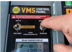
4. **Shutting Down: The sign MUST be BLANK when towed.** Blank the sign using the BLANK SIGN switch on the VMS Control Panel.
