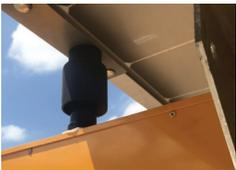
5. If a Manual Solar Tilt/Rotate (STR) system is fitted, rotate and lower the solar array back into park position. Undo the lock using the handle. Use either the handle or the drill adaptor bit. Make sure the holding cups are on the aerials when lowering and sit all the way down.
