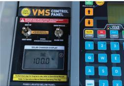
The Amps will be high when the solar panel are facing towards the Sun, as the Battery charge level goes up the Amps will decrease.
