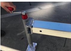
6. Retract the Wind down Legs up and slide in the outriggers on all four sides.
