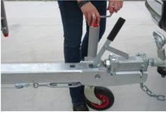
8. Use the Jockey wheel to lower the tow coupling onto the tow ball. Ensure the tow coupling fits snugly onto the tow ball of the towing vehicle. This is discussed further in this manual.
