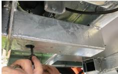
3. Remove the cover screw using the M6 TOOL BIT from underneath the actuator (keep it safe to put it back in again afterwards).
