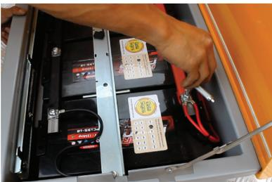
The batteries are secured using a +Ve and -Ve Bus Bar and held with unique security bolts which can only be undone using the DataSigns T-Tool.
