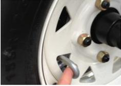
1. Remove the security chains from through the wheels.
