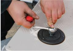
1. Use the handle to lock and unlock the cap.
