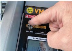
3. Lower the Sign Head using the Hoist Down switch on the VMS Control Panel in the VMS Control box.
