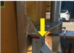
2. Undo the Mast Brake to lower the Sign Head. Lower Sign Head into transport cradle as shown.
