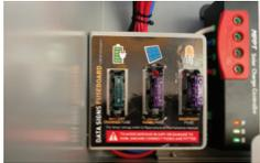
1. The power supply **MUST** be disconnected during manual lowering operation, pull out the **ALL** the fuses found under the shelf in the VMS Control Box.
