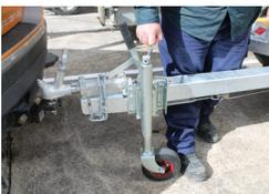
6. Undo the safety chain from the vehicle and wind the jockey wheel to allow the tow coupling to be free of the vehicle tow ball.
