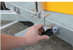
13. Plug the tow cable into the plug on the trailer and the towing vehicle.
