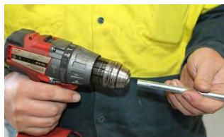
The electric actuator is used to raise and lower the Sign Head. In the event of low voltage, defective batteries or actuator failure, the electric actuator can be manually lowered.
