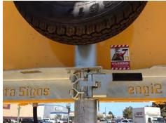
11. **Setting up for Operation:** Raise the Sign Head using the Hoist Up Switch to clear the cradle and the control box open lid. Rotate the Sign head to face oncoming traffic and LOCK the mast brake again.
