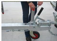
7. Use the Jockey wheel to lower the tow coupling onto the tow ball. Ensure the tow coupling fits snugly onto the tow ball of the towing vehicle. This is discussed further in this manual.
