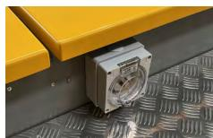
To charge the batteries, plug the power cable into 240V Mains power.
