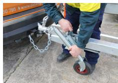
9. Wind up the jockey wheel and lift to slot into position. Make sure the jockey wheel does not move once in the towing position.
