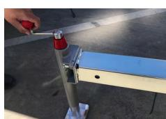
5. Retract the Wind down Legs up and slide in the outriggers on all four sides.
