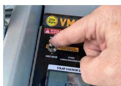
3. Lower the Sign Head using the Hoist Down switch on the VSL Control Panel in the VSL Control box.
