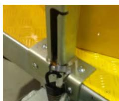
4. Slide lock-pin lever into bracket to hold and secure in place with a lock.
