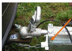
10. Ensure the Reversing lock on the tow coupling is released before travelling, as shown.
