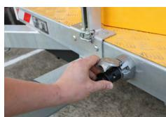
12. Plug the tow cable into the plug on the trailer and the towing vehicle. Check the trailer lights are functioning correctly.
