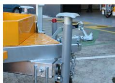
6. Pull the spring pin and rotate the wind-down legs upside down, ensuring the spring pin goes back in to lock the wind-down leg in the upwards position.
