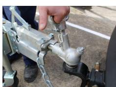
4. Unclip the tow coupling. Let the clip rest as shown.
