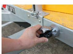
5. Undo the trailer cable and store this under the shelf in the VSLS Control box.
