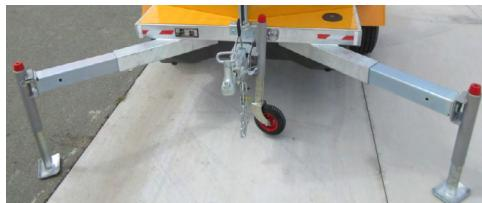
1. Ensure the two front wind-down legs are lowered in the down position to prevent tipping whenever the drawbar is retracted.
