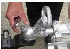
3. Using a flat-head screw driver on the slot on top of the pin, turn until tight, and then loosen very slightly. This will pull the coupling forward onto the tow ball and grip it.
