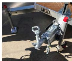
2. Release the wheel brake. The jockey wheel should only just touch the ground so there is no upward pressure on the drawbar; you should be able to wobble the drawbar. This ensures the pin can move freely.
