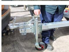
6. Undo the safety chain from the vehicle and wind the jockey wheel to allow the tow coupling to be free of the vehicle tow ball.
