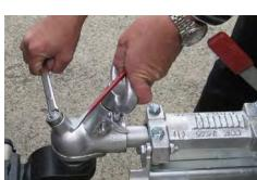
6. Note: when towing, ensure the reverse-lock is not engaged. Push out of the way, as shown.
