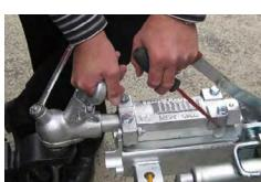
5. Tighten the locking nut firmly.
