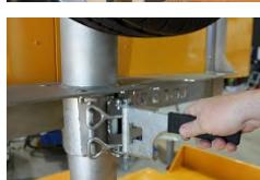
6. Stop winding when lowered to the base.
