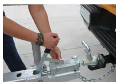
11. Release the hand brake if this is still engaged.
