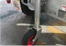
1. The Dolly wheel on the Rear trailer should be faced outwards to couple the trailers together.
