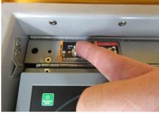
7. Press and hold the SLAVE LINK switch to the JOIN /IN position to join the trailers together using the actuator.
