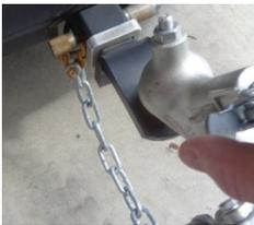
3. Unhook the tow coupling on the Front trailer from the Vehicle to allow for levelling. Leave the security chains attached to the Vehicle.
