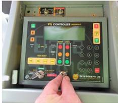
1. Gain access to the Control box. Turn the ON/OFF key-switch on the Controller to OFF position to turn the PTL's off.
