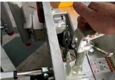
4. Pull out the locking pin. Move the trailers until position as shown. The link actuator should be fully extended at this point.
