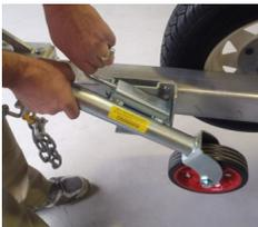
2. Lower the Jockey wheel on the Front trailer and make sure it is locked into place with the pin. Use the jockey wheel to assist with Unhooking from the Vehicle and to level out the Front trailer.
