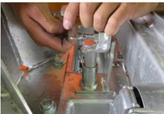
5. Push the trailers together, insert the Locking pin back in so that it drops back on the front trailer tow section.
