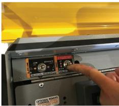
3. The Control box contains the Hoist UP/DOWN switch.
