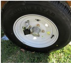
4. Pull the wheel chains through the wheel and padlock to secure.
