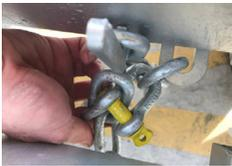
9. Use the safety chains from the Rear trailer and connect to the Front trailer as shown, lock on to the Front trailer safetychains using the D-links.
