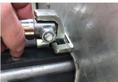
6. Fully extend the actuator and push down onto the lip on the Front trailer.
