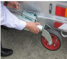
5. Lower the Jockey wheel on the Rear trailer and use this to level out the trailer. Level out both the Front and Rear trailers as much as possible. *Use the Water Level Marker on the Front trailer draw bar to assist with this process.*
