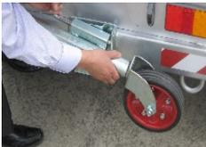
11. Raise the Dolly wheels up on both the Front and Back trailers, and ensure they lock into place.
