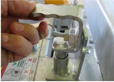
8. When trailers are joined, the locking pin will drop into place. Use the spring pin as shown to lock the pin into place. It can be further secured with a lock if necessary.
