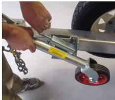
4. Ensure the Dolly wheel is lowered and locked into place with the pin.
