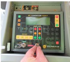
5. Turn the Controller on by turning the key-switch to the ON position.
