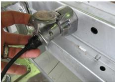
10. Plug in the trailer light cable onto the plug on the back trailer.
