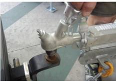
2. Unhook the tow coupling from the vehicle and lower the Dolly wheel. Leave the security chains attached. Use the Dolly wheels on the Front and Rear trailers to level out and align together.
