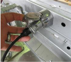
1. Remove the Trailer Light cable from the Rear trailer. We recommend storing the cable in the Rear trailer Control box, or connect it onto the Front trailer if it has to be towed to another location.
