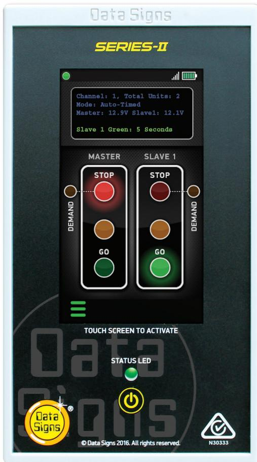
The Optional Remote Control is used by the operator to control traffic flow when the Master Controller has been set to Manual mode either in Shuttle or Plant-Crossing operation. It is recharged by placing it in the cradle in the Master Control box.
