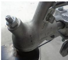
5. Hook the trailer up to the towing vehicle. Attach the safety chains using D-links. Attach the trailer light cable.
