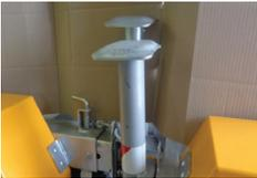
3. Retract and position all Jackstands as shown. i.e. For the Jackstands in the middle of the trailers, the front Jackstands are in a higher position than the rear Jackstands.
