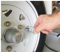
3. If chains are locked through wheels, unlock and pull chains through and secure onto the trailer. Do this on both wheels.
