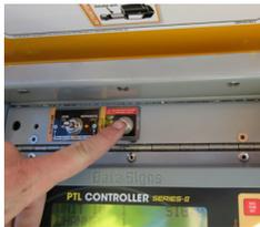
2. Lower the Traffic Light using the Hoist DOWN switch located in the Control box.
